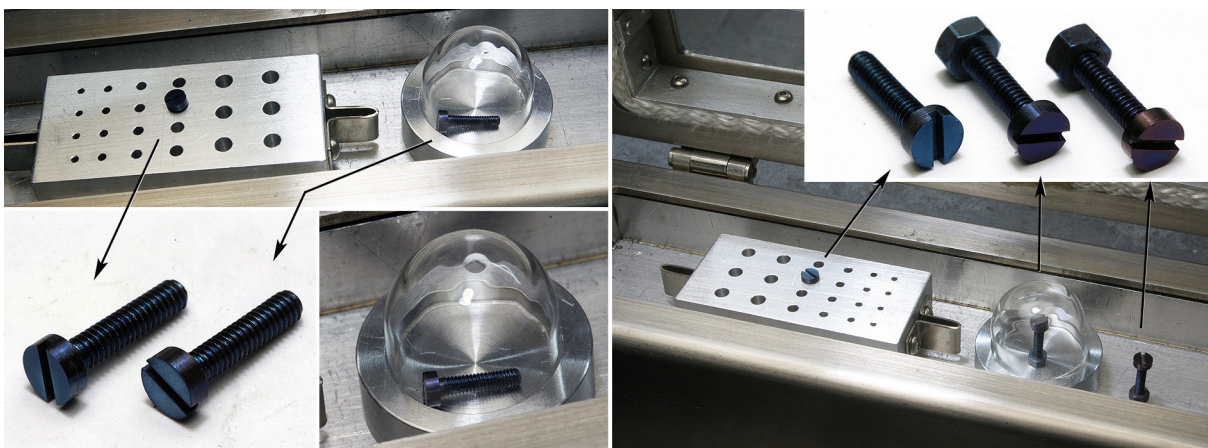
Figure 2.18: Comparison of the results of bluing screws using a block and chamber with the screws in differing orientations
