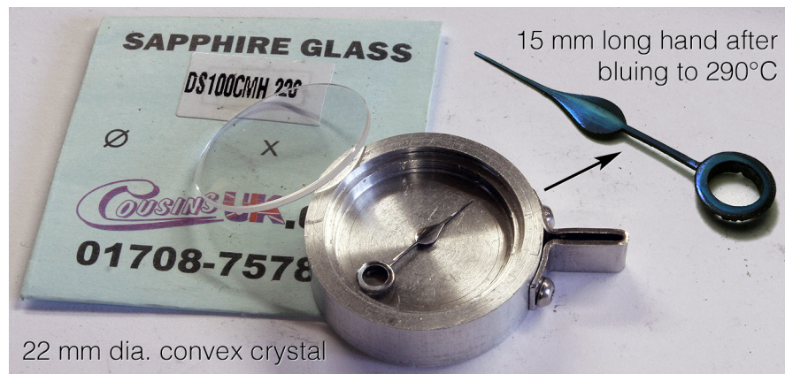
Figure 2.19: A crystal chamber made from a watch glass
