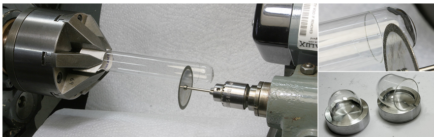
Figure 2.17: Cutting a borosilicate chamber from a test tube
